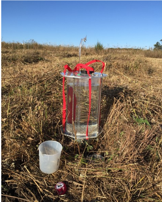
Figure 8. Setup for the Cornell Sprinkle infiltrometer.
