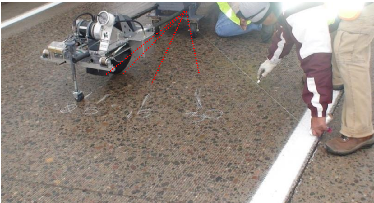
Figure 34 CT-342 Measuring Friction at Various Angles at MnROAD 17
