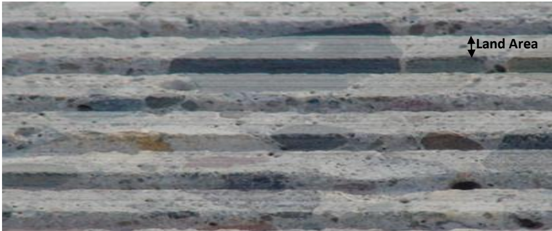
Figure 10- Photo of Purdue Negative Texture Profile (e.g. NGCS) and Land Area
