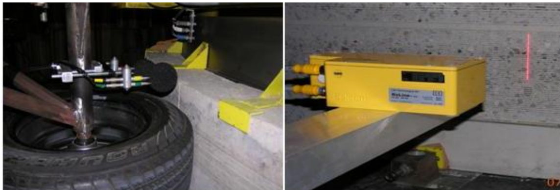
Figure 2- OBSI and RoLine™ Test Equipment Mounted to TPTA 2
