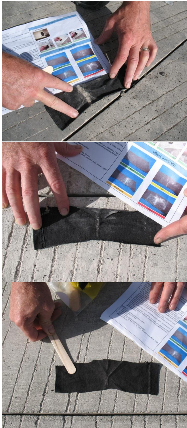
Figure 21. Wipe test results from field testing. Top to bottom: Not cleaned; powerwashed; and powerwashed and sandblasted.
