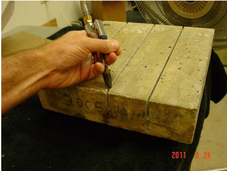
Figure 2. Sawcut joint being cleaned and dried with compressed air.
