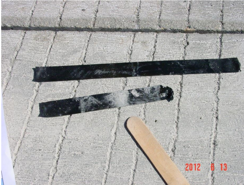
Figure 22. Tape test results from field testing showing cleaned (top) and uncleaned (bottom) joint test results.
