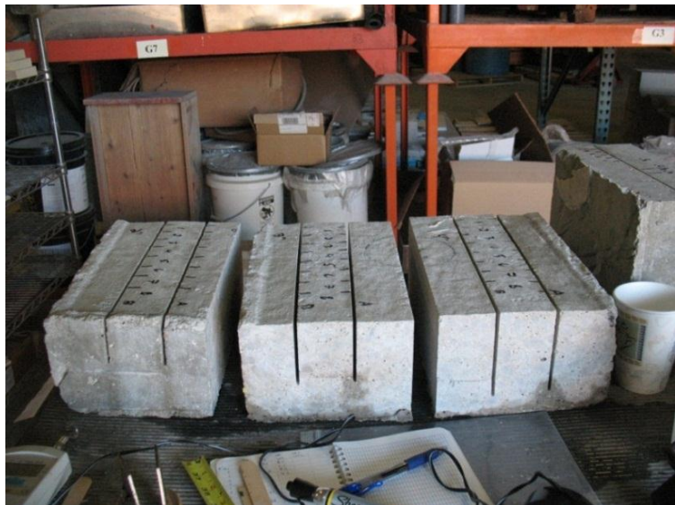
Figure 1. Typical sawcut joints used during laboratory testing.
