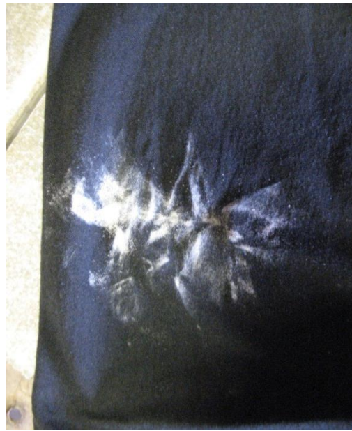
Figure 10. Dark cloth wipe test on uncleaned joint.
