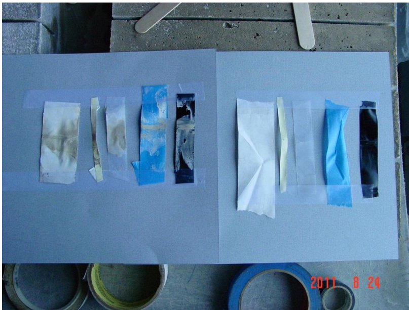
Figure 12. Tape test results for uncleaned (left) and cleaned (right) joints.
