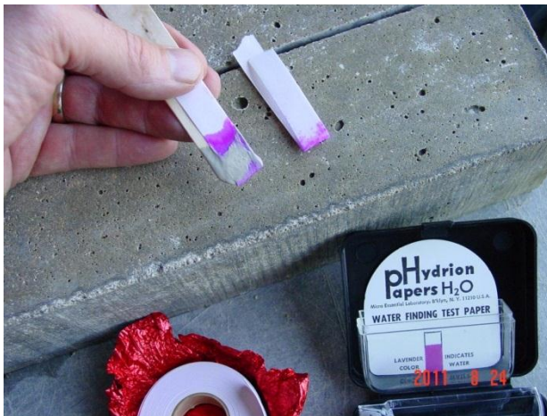
Figure 6. Moisture sensitive paper test. Purple indicates the detection of moisture.
