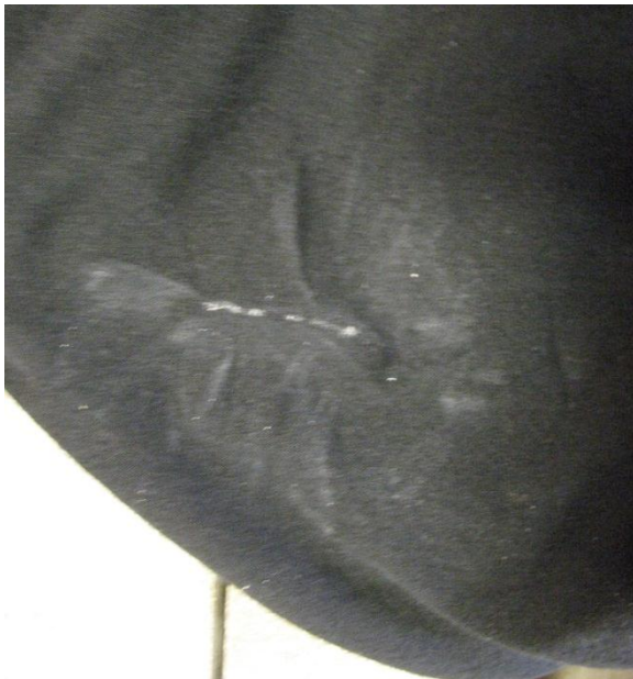
Figure 9. Dark cloth wipe test on cleaned joint.
