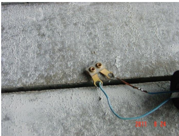
Figure 3. Relative humidity probe modified to fit into sawcut joint.
