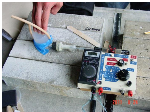
Figure 4. Relative humidity probe test.
