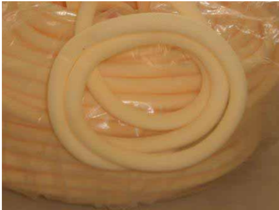
Figure 5 7/8 Inch Denver Foam Used as Backer Rod for Wide Joints
