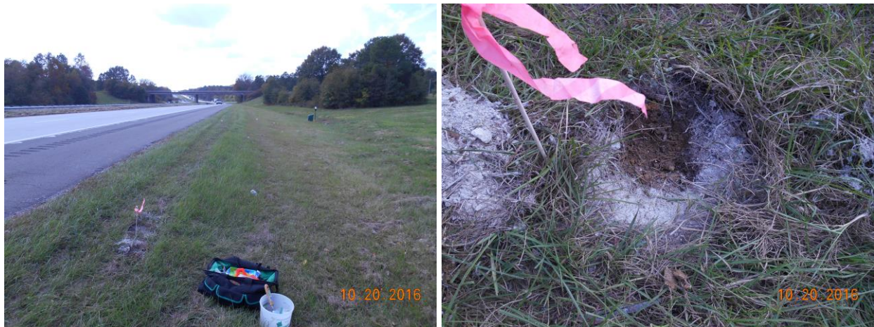
Figure 6. Soil sampling location on shoulder (left) and sampling hole with DGS cleared (right).
