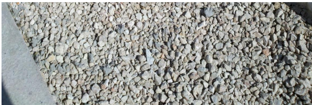
Figure 33 Open Graded Granular Subbase Used for Test Program.
